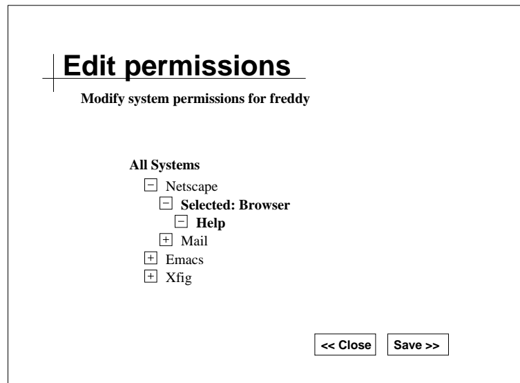
Figure 3.23: The permission tree makes it possible to modify a given type of permissions for a user by selecting and deselecting systems in the tree.
