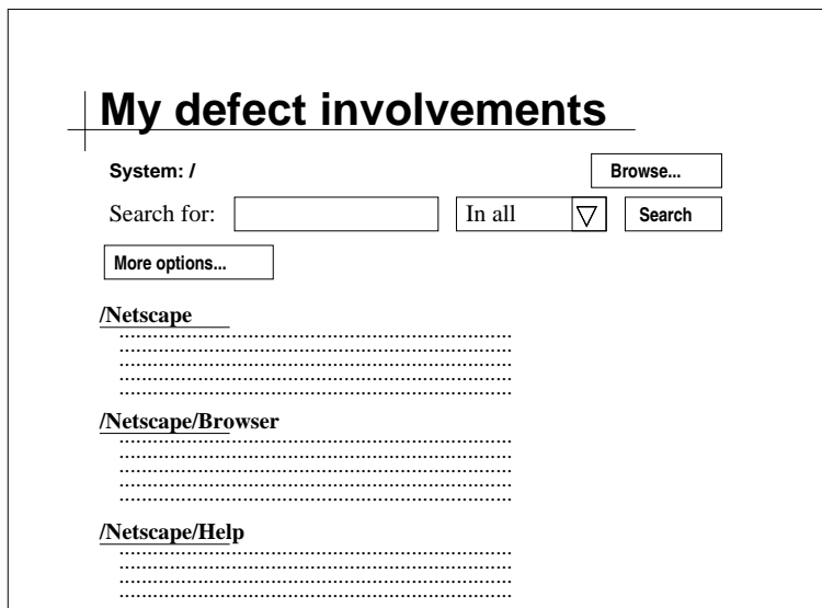
Figure 3.17: My defect involvements is designed to give a good overview of the reports that the actor is affiliated with. Selecting one of the defects will forward the actor to the view report page.
